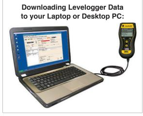
You can download Levelogger readings from your Leveloader to your desktop or laptop PC, using a USB or RS232 Communication Cable and Levelogger Software Version 4.0 and higher. You can also create and save up to 10 customized Levelogger settings files for transfer to Leveloggers in the field.
