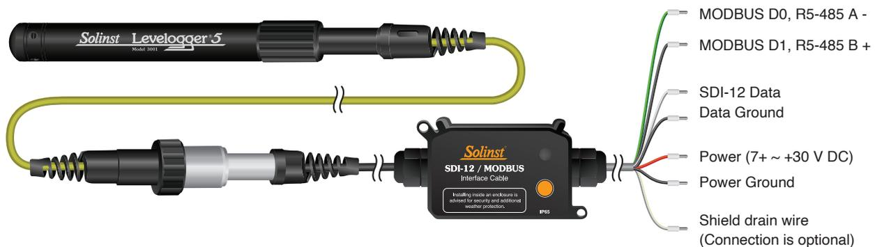
**Figure 3-1 Datalogger SDI-12 Wiring Overview**
