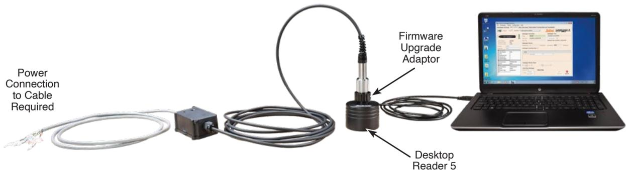
Figure 6-1 Firmware Upgrade Setup
