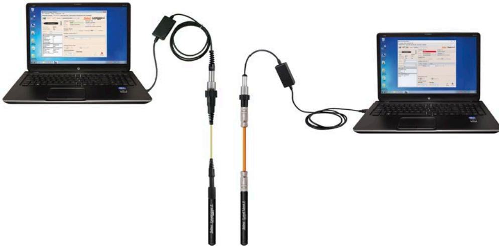
Figure 3-1 Communicating with Levelogger Software
