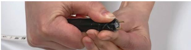
6. Use your fingers to install the new o-rings in the grooves. You can lubricate them with a bit of water if required.
