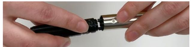
11. Line up the indents in the probe with the grooves in the tape seal plug. Push the probe past the o-rings, then twist the probe clockwise until the probe seats on the tape seal plug.
