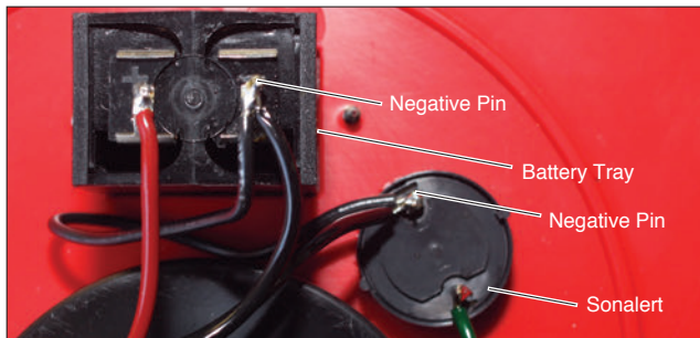
Unsolder the Wire Connections and Note the Pin Positions
