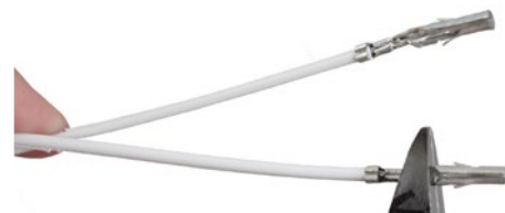
Cut the Pins on Each Tape Lead in Half (as shown)
