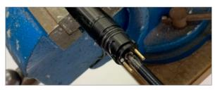
5. Use pliers to pull out the two brass tubes and the black disk from the tape seal plug.
