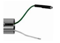
2. Use the Molex Crimp Tool (2 mm position - see photo at top) or suitable pliers to connect the crimp terminal to the wire. Tug the crimp terminal to ensure it is securely attached to the wire.
