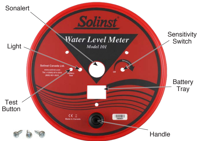
101 P7 Replacement Faceplate Assembly indicating the location of the components (comes with Handle Assembly attached and 3 Phillips screws)
