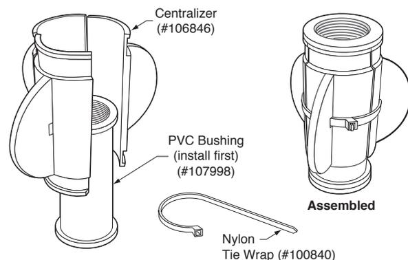
Figure B - 3.9" (99 mm) Centralizer Assembly
