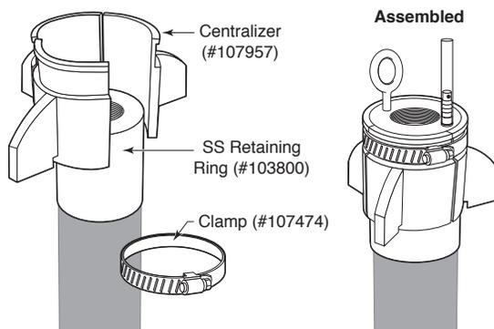
Figure A - 1.8" (46 mm) Centralizer Assembly
