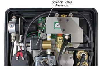
Push down on the fittings to remove the three black tubes from the Shuttle Valve Assembly, and the two clear tubes from the Solenoid Valve Assembly (photo shows black tubes removed).
