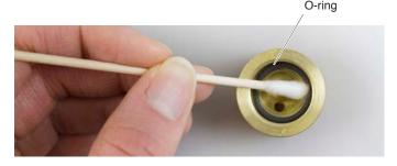
11. Ensure the o-ring is properly seated inside the brass fitting. Insert the magnetic plunger back into the Solenoid Valve Assembly, and screw the brass fitting back onto the Assembly.
