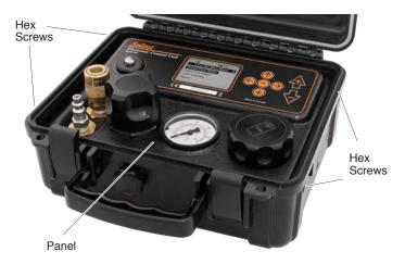
Remove the panel from the Control Unit and flip it over to access the Solenoid Valve Assembly.
