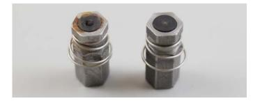
10. To clean the Assembly, use a cotton swab and distilled water to clear any debris and dirt from inside the brass fitting, around the o-ring, steel fitting and from the magnetic plunger.
