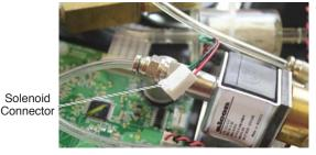
6. Remove the tubing from the three fittings on the Solenoid Valve Assembly, by pushing on the "grasping ring" on the fitting (to release tubing) and pulling the tubing out.
