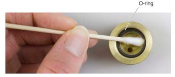
11. Ensure the o-ring is properly seated inside the brass fitting. Insert the magnetic plunger back into the Solenoid Valve Assembly, and screw the brass fitting back onto the Assembly.
