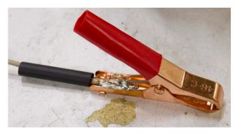
12. Slid the grips over the heat shrink and onto the handles of the new clins
