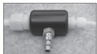
*Tighten the compression fitting nut*
