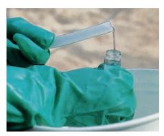
Low flow methods allow the collection of high quality, representative groundwater samples in 40 ml glass vials for VOC analysis.
