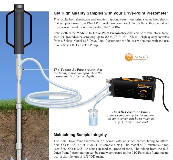
This setup maintains sample integrity from the Drive-Point Piezometer tip to the sample discharge at surface, even when inexpensive carbon steel extensions are used. Connecting the tubing from the Drive-Point Piezometer tip to the pump head prevents sample water from contacting the steel extension rods of the 615 Drive-Point Piezometer during sampling. The piezometer tips and screens are made of high quality stainless steel, allowing a "clean" sample.
