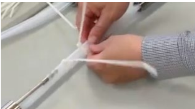
Keep tubing from twisting before adding extension.
