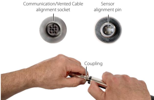
Connecting Sensor to Communication/Vented Cable
