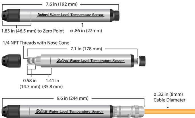
Water Level Temperature Sensor Dimensions
