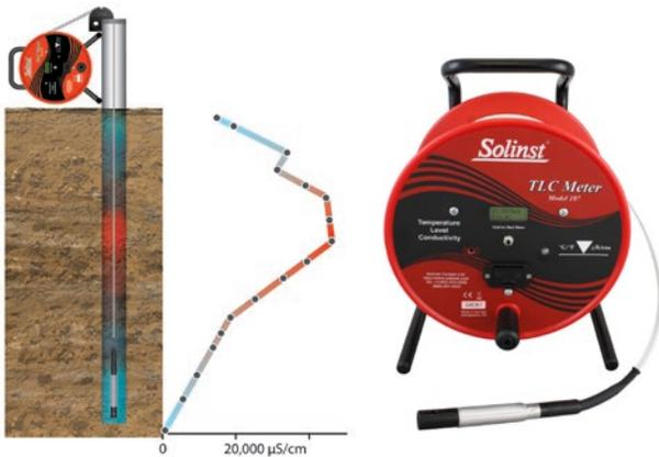
The probe is attached to high quality flat tape for depth readings, which is indicated by a light and buzzer. The tape is accurately laser-marked each millimeter or 1/100 ft, in lengths up to 300 m or 1000 ft. The probe and tape are mounted on a sturdy reel making operation easy. Conductivity and temperature measurements are displayed on an LCD display.
