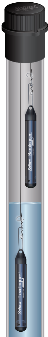
Figure 10-12 Levellogger and Barologger in Well
