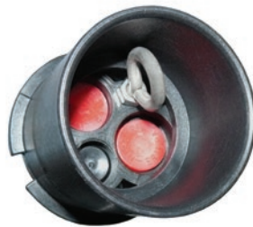
Bottom View shows eye- bolt used to secure pumps and Levelloggers
