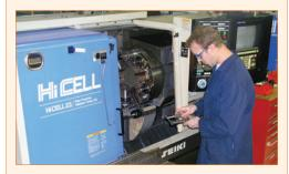
Our production area features three CNC machines (Computer Numerical Control). They allow precision machining of stainless steel, PVC, Teflon<sup>®</sup>, Delrin<sup>®</sup> and other materials, which are used to produce many of the components for our products, including Levelogger housings, water level meter probes, pumps, multilevel system components, and drivepoints.
