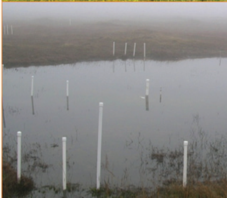
Top: Vernal pool wetland during spring season with slotted PVC pipes containing Levelogger Juniors at a research site near Sacramento, California
