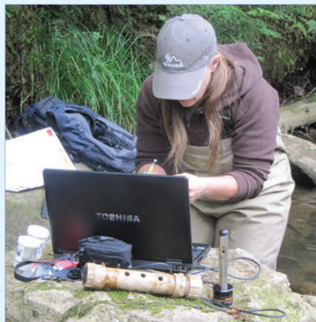
LTC Levellogger Junior dataloggers are calibrated in the field before deployment
